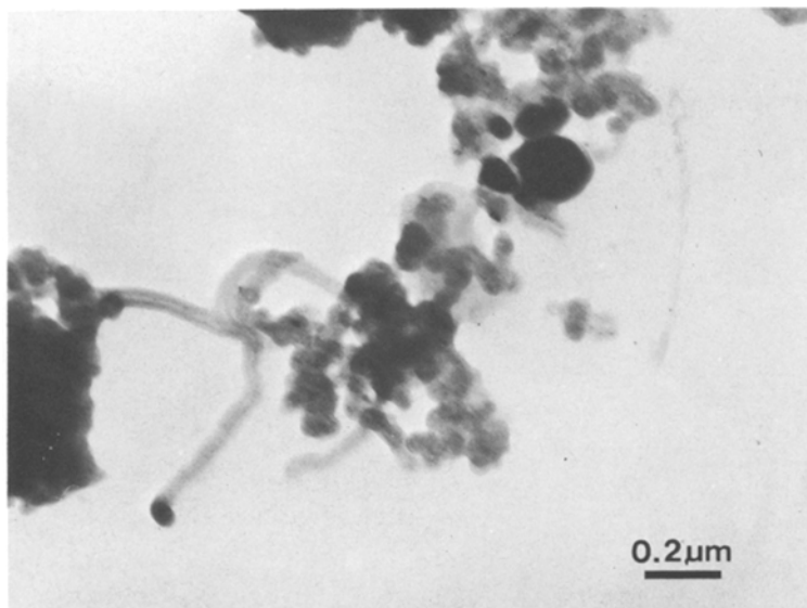
Figure 2 Microstructure of fibrous carbon dispersed with particles of cementite prepared from DVB-14.4 mol%VF by pressure pyrolysis.
